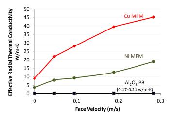
Figure 2. Effective radial thermal conductivity of Cu MFM, Ni MFM, and  $Al_2O_3$  Packed Bed (PB) as a function of face velocity.
